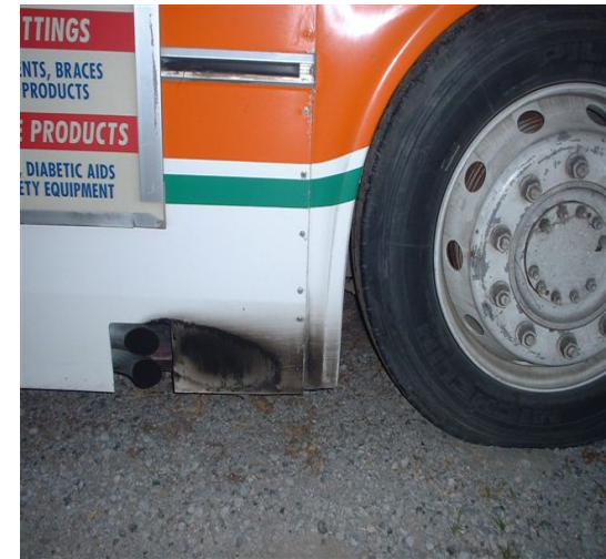
After Tadger Installation September 04, 2002
